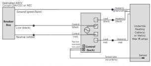
NOTE: All electrical work must be performed by a qualified electrician in accordance with local building & electrical codes and The Canadian Electrical Code, part 1 in Canada or the National Electrical Code in the USA, especially Article 424, Part V of the NEC ANSIINFPA 70.
